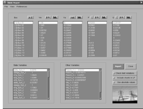
Fig. 6. GUI for power flow reports. The results refer to the IEEE 14-bus test system.
